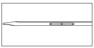
If the oil is below the cross-hatched area at the tip of the dipstick, you will need to add at least one quart/liter of oil. But you must use the right kind. This section explains what kind of oil to use. For engine oil crankcase capacity, see *Capacities and Specifications on page 452*.
